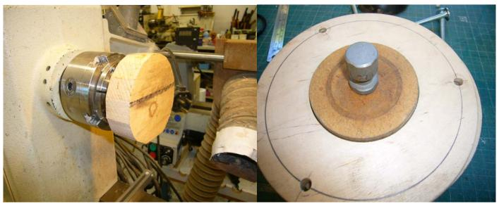
I start with a blank about 3.5" (30mm) diameter on a screw chuck with a backing disc the same diameter as the recess in my doughnut chuck front ring. I then turn or use a sphere jig to get the dome shape and diameter to match the backing disc. I normally put some wax on the screw chuck so I can unscrew the finished piece
