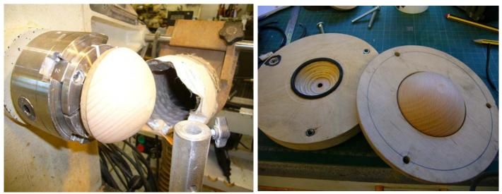
I turn the inside with a bowl gouge to a wall thickness of about 3/32" (2-3mm I make the step in the front ring to this dimension.
